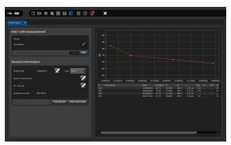
Trend analysis (insulation testers and micro-ohmmeters)
